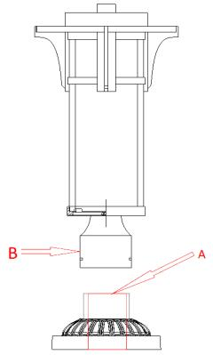
THERE IS ABOUT 70mm HOLE ON THE BASE STEM (ARROWED A AND MARKED RED) WHICH IS THE CABLE ENTRY AND THE IP BOX SITS IN THE AREA MARKED B TO BE CONNECTED TO COMPLETE THE CIRCUIT.
