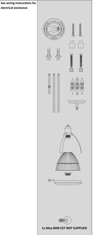
Help line +44 1420 82377 IT IS RECOMMENDED THAT LIGHTS ARE INSTALLED BY A QUALIFIED ELECTRICIAN
