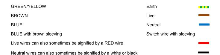
CLASS I Luminaires (Earthed) - Connect the brown wire from the luminaire to the supply live wire (red or brown). Connect the blue wire to the supply neutral wire (black or blue). Connect the green/yellow wire to the supply earth wire (green/yellow) or connect the supply earth to the luminaire earth terminal marked:
