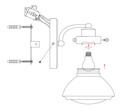
If this product is being installed in a bathroom or a location where the product will be exposed to high levels of moisture, you should apply a silicone seal around the back-plate/canopy.
