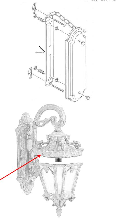
TO CHANGE THE BULB PLEASE UNSCREW TWO SCREWS ON THE SIDES (ARROWED) TO RELEASE GLASS SHADE
